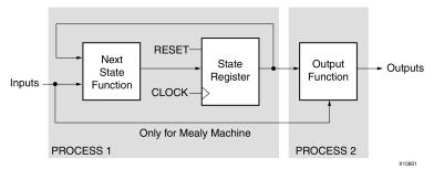
A Finite State Machine (FSM) With One Process can be described with three processes using the FSM decomposition shown in the following diagram.
